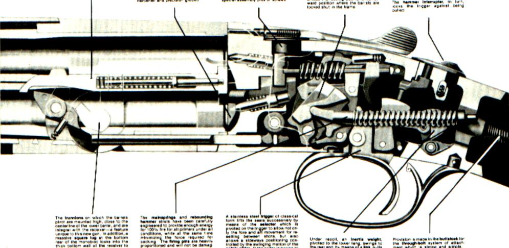
Figure 1 — MECHANISM CROSS-SECTION
